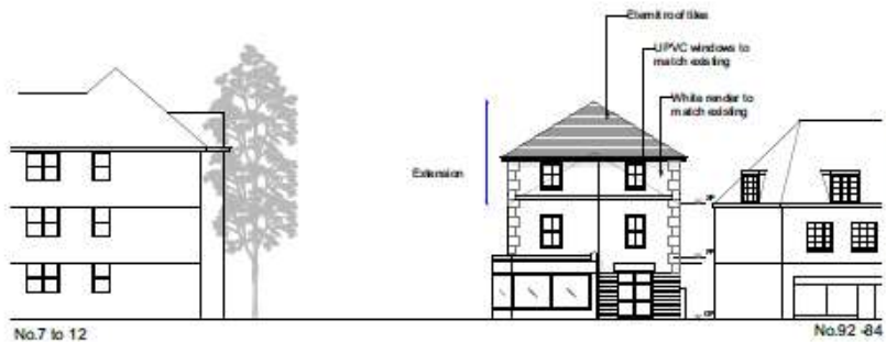
FRONT ELEVATION (Facing Brighton Road) 1:100 @ A1
